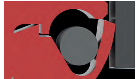
The gasket lip is in contact at low speed or stop – maximum protection
