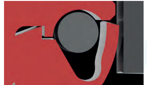
The gasket lip lift-off if speed is rising – gap shows up
